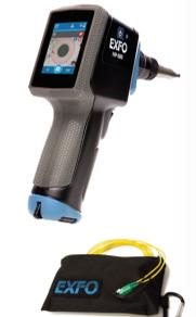
The launch/receive fiber resides between the equipment (OTDR and/or iOLM) and the FUT
