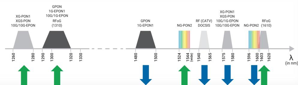
Example of a next generation PON network using GPON, RF video and XGS-PON overlay.
