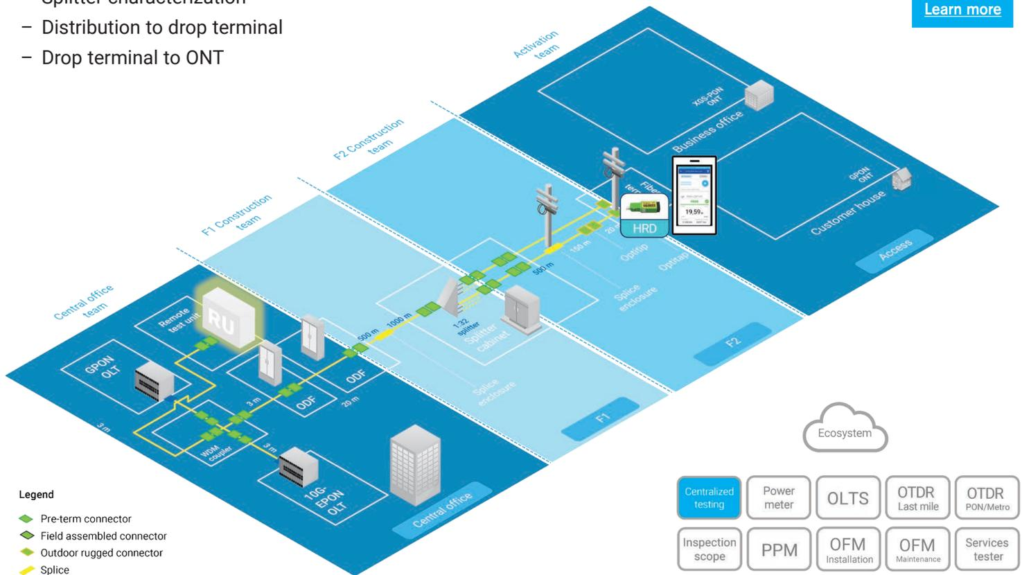
The use of field portable testers is vital for fully characterizing, installing, troubleshooting the optical link from customer premises to the OLTs in the exchanges or central offices.
