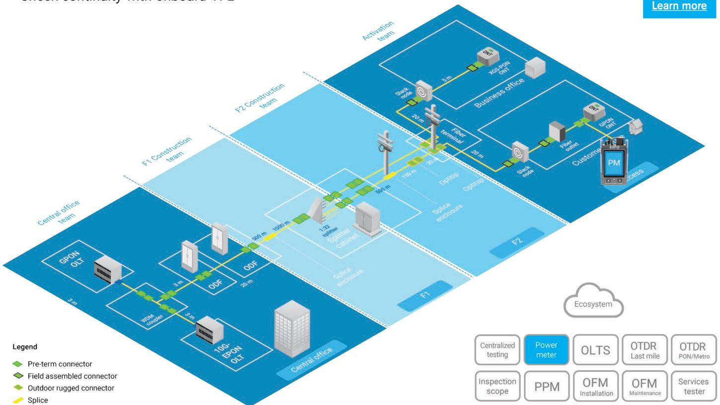
After the fiber is installed and prior to FTTH service activation, the power at the optical network terminal (ONT) socket has to be checked. It is crucial to ensure that there is enough power for the ONT to function.
