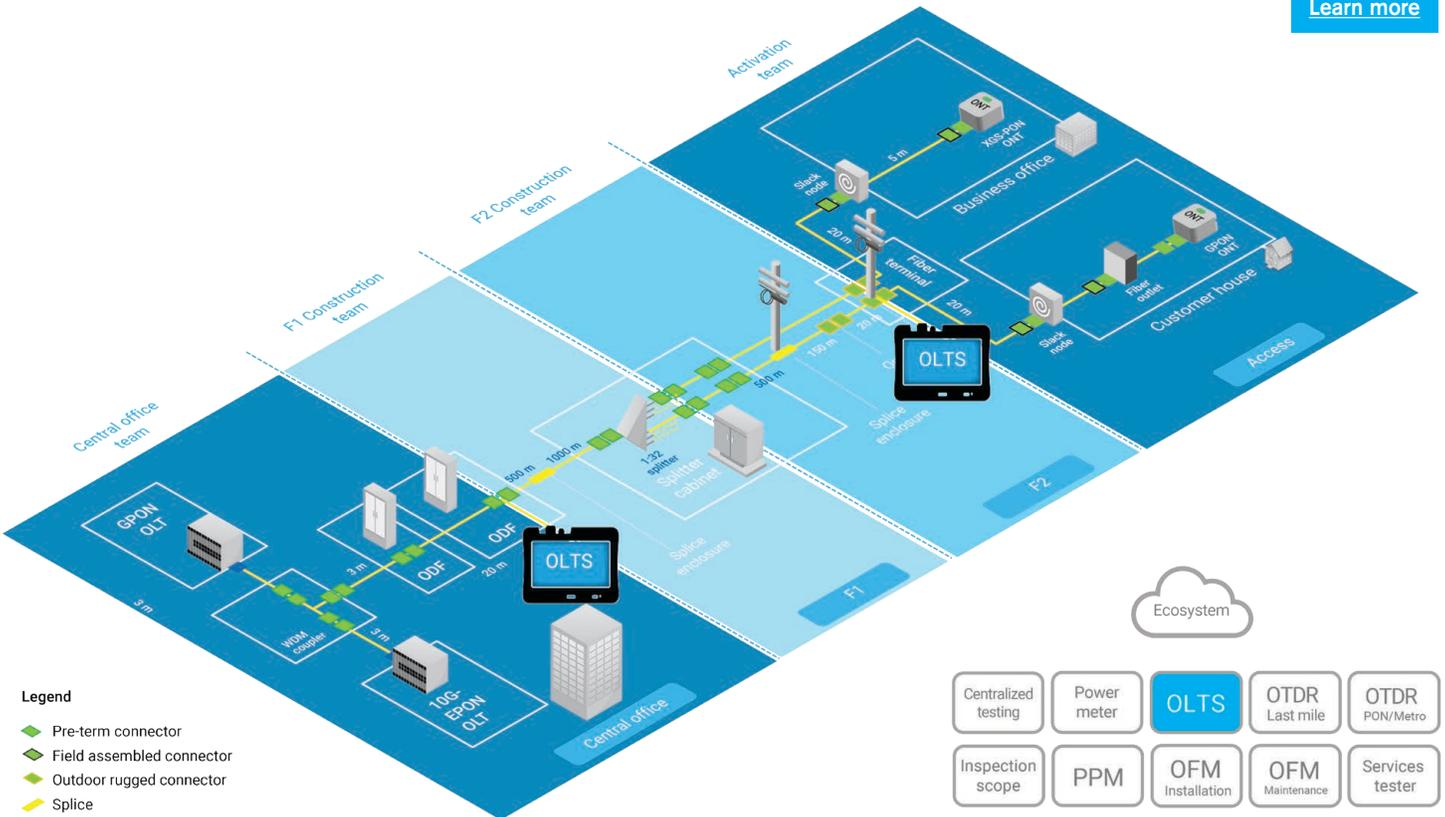
Once the splitter(s) have been installed, it is important to quantify the total loss and confirm whether it is within the loss budget.
