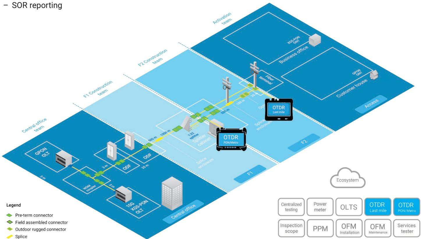
On any FTTH construction job, it is critical to have the right tools to fully characterize cables before moving on to the installation phase. An optical time-domain reflectometer (OTDR) is an absolute necessity.
