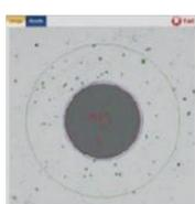
Contaminants in a connection will impact reflectance and loss.
