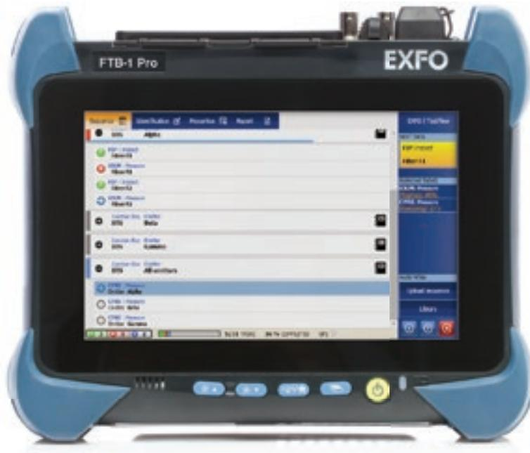
Figure 77. Example of test results tracked within the TestFlow application on the FTB-1 Pro test platform.
