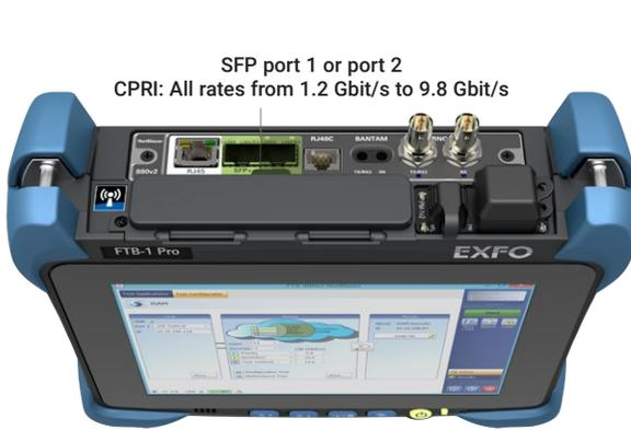
Figure 18. CPRI interfaces on the FTB-870 V2/FTB-880 V2 modules
