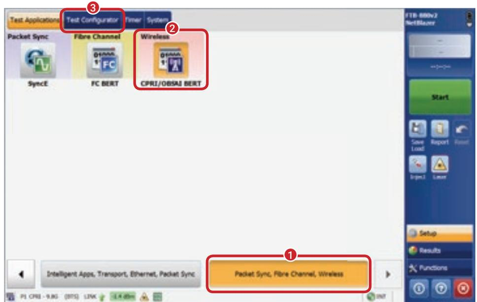
Figure 22. Starting the CPRI Test Application
