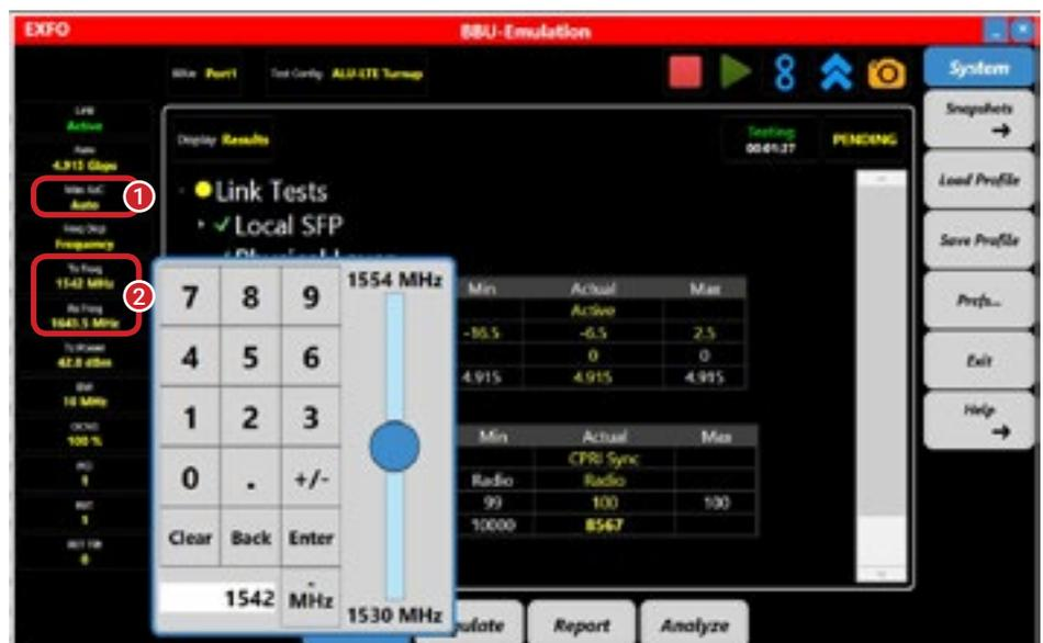
Figure 58. BBU emulation Tx frequency
