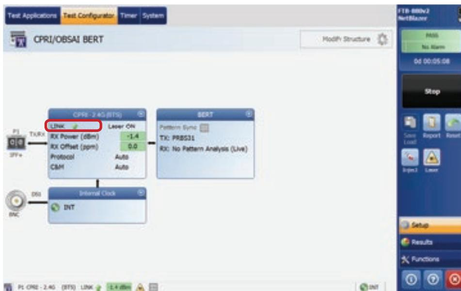
Figure 49. RTD Measurement: CPRI link-up with RRH
