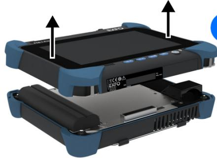
Pull on the battery's tab to free it from its socket.
