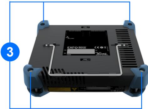
**4** While holding the front panel and the module firmly together, turn the unit over, and position it so that the module rests on a flat surface such as a table.
