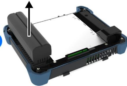
Slide in the new battery (poles facing down and pointing to the same side of the case as the mating connector).
