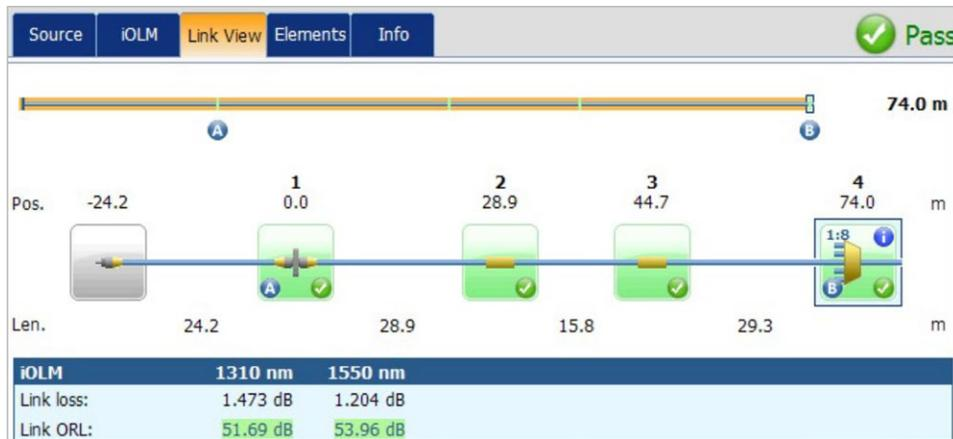
Figure 3. Test Pass—Last mile loss and ORL are within specifications. Splitter presence is confirmed, matching expected ratio and there is continuity to feeder. Last Mile installation is guaranteed.
