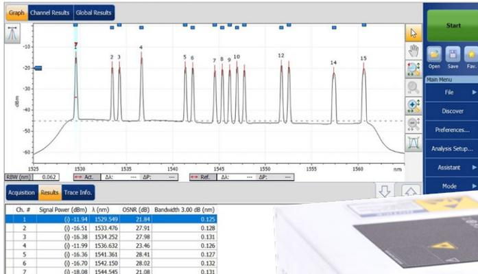
Compact OSA for DWDM, CWDM, and DWDM over CWDM networks.
